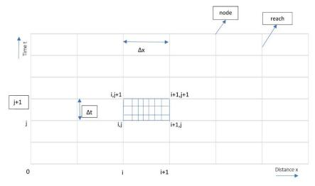
Fig. 1. The distance-time grid to developed implicit finite difference scheme.
