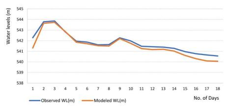
Fig. 7. Validation water level profiles (stages) at Phulgaon gauging station (from 20 July 2005 to 8 August 2005).
