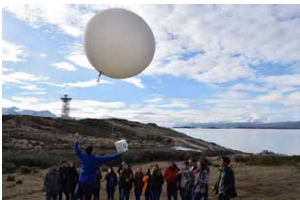
Figure 1. Ozone observation at Ushuaia, Argentina. Ozonesondes measure ozone and meteorological variables at different altitudes as the sonde ascends, until the balloon bursts. (Source: Lino Condori)
