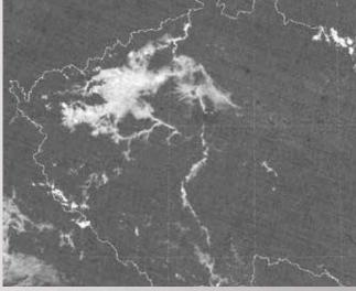
Detection of early morning fog over the Czech Republic based on current Meteosat Second Generation imagery (left) and with proxy data simulatin
