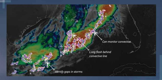
This image taken by the US GOES Geostationary Lightning Mapper (GLM) instrument shows lightning activity in white-blue-magenta colours along a convective storm line (yellow-orange-red shades in background infrared imagery) over the Gulf of Mexico. The GOES GLM is a precursor to the MTG Lightning Imager.
