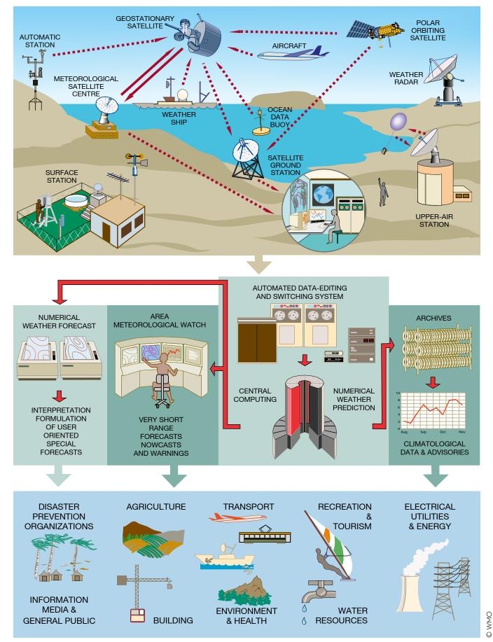
The planned integrated structure of the World Weather Watch with the Global telecommunication System (GTS) and the Global Data Processing System (GDPS) for the collection, processing and exchange of observations from the surface and space-based components of the Global Observing System (GOS).
