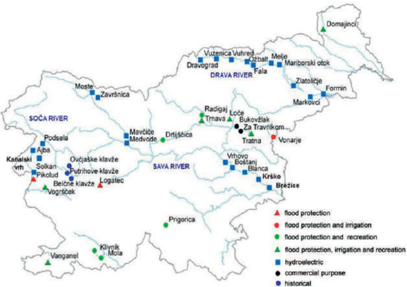
Fig. 3. Large dams in Slovenia [SLOCOLD]
