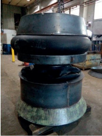
Fig. 3. Submersible closing facility during manufacture [PPH-1200 technical documentation; K+K servis Ltd.]
